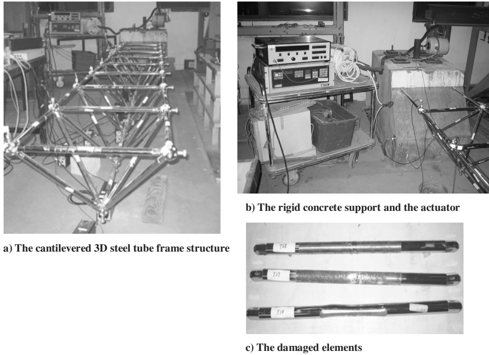
Fig. 4 Experimental setup and the damaged elements of the nine-bay frame structure.
